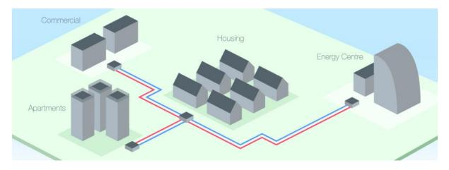
Figure 5: Centralised/ Communal Heating System
