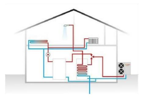
Figure 6: Air Source Heat Pump Diagram
